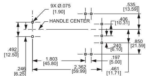
**Printed Circuit Board Mounting Terminal Type "L"**
