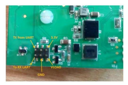
The custom cabling connect the USB/TTL cable, power supply unit and Radon Module:
