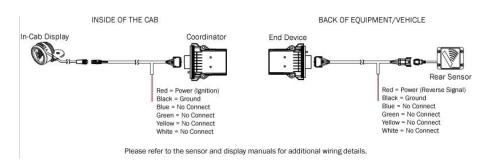
Figure 1 -Single Sensor with Display, System Wiring Connections. Please refer to your system specific wiring diagram for additional specifications.
