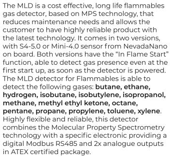
It is also equipped with two relays (Alarm 1 and Alarm 2/Malfunction) to offer a clean signal that can be managed in an intuitive way. It comes with 1,5 or 3 meters cable.
