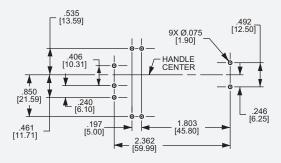
Note: Tolerance ± .015 [.38] unless noted. Dimensions in brackets [] are millimeters.
