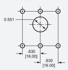
Note: Tolerance ± .015 [.38] unless noted. Dimensions in Brackets [ ] are millimeters.
